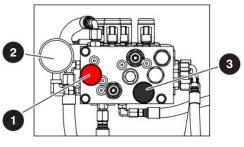
Figure 23 Brake Manifold
