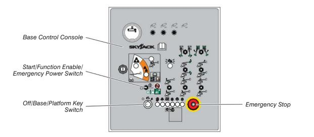
4.3-4 Test Start/Function Enable/ Emergency Power Switch and All Boom and Platform Functions
