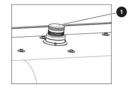
Figure 18 Flashing Amber Light
