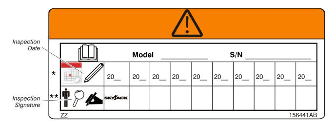
**Figure 33** This decal is located on the control compartment cowling. It must be completed after an annual inspection has been completed. Do not use the MEWP if an inspection has not been recorded in the last 12 months.
