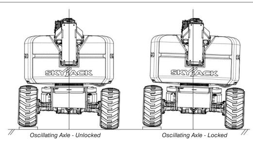
4.3-23 Test Oscillating Axles
