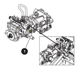
Figure 22 Drive Bypass Valve
