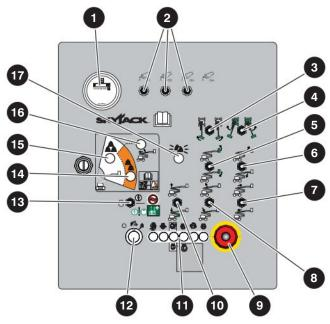
Figure 07 Base Control Console
