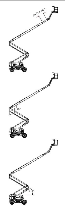
Figure 10 Elevated Travel Position (any of the boom positions shown)
