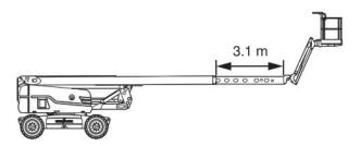
Figure 12 Fly Boom Extension into Low Capacity Zone
