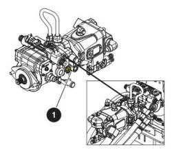
Figure 21 Drive Bypass Valve
