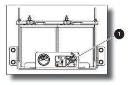
Figure 05 Main Power Disconnect Switch
