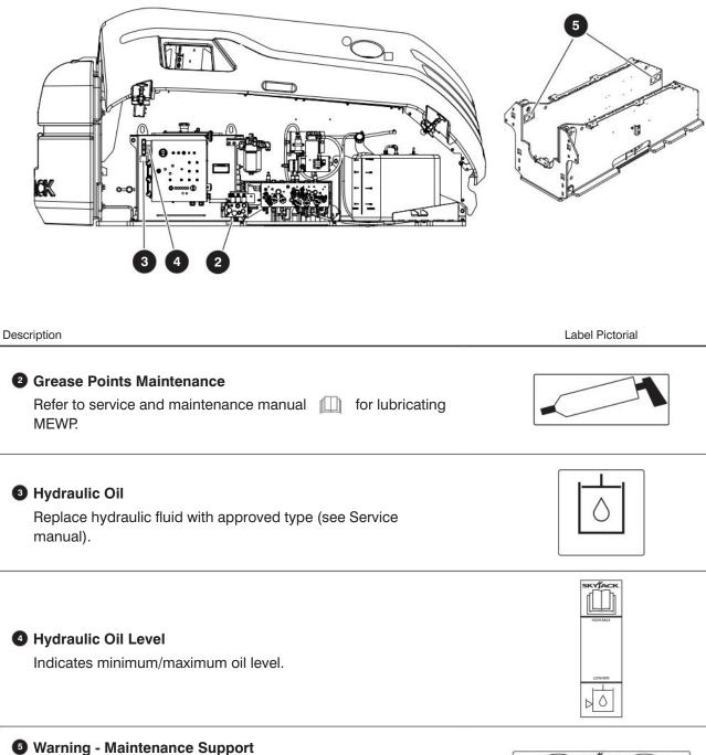
Do not enter the space beneath the work platform or extending structure during maintenance unless a means of structure support is in place. Refer to Service manual for instructions regarding machine power isolation and structure support during maintenance.
