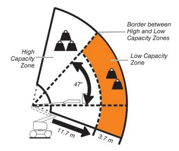
Figure 11 High and Low Capacity Zones
