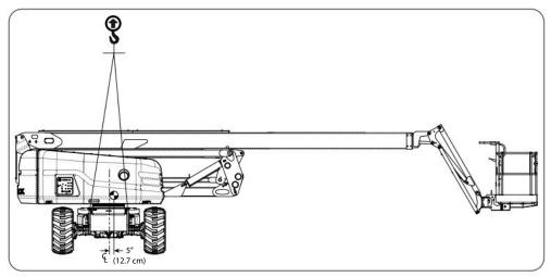
Figure 29 Center of Gravity
