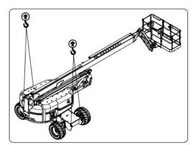
Figure 28 Lifting Points
